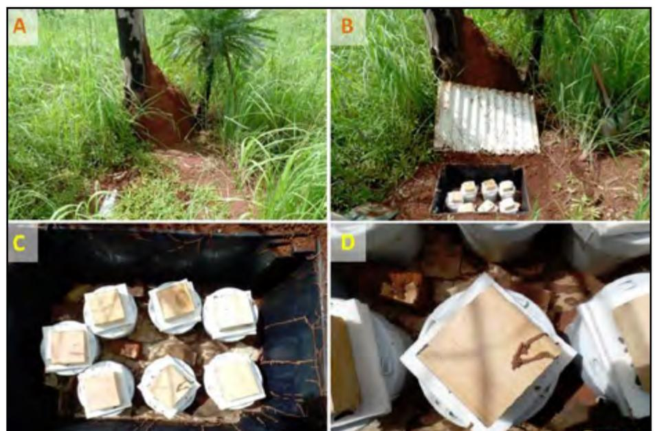
Figure 1: Greenzone field trial showing (A) position of trial next to known termite activity; (B) at inspection, the covering soil and corrugated steel cover are removed; (C) interior of a buried box with experimental Greenzone units intact; (D) close up of Greenzone ant cap barrier and test wood
